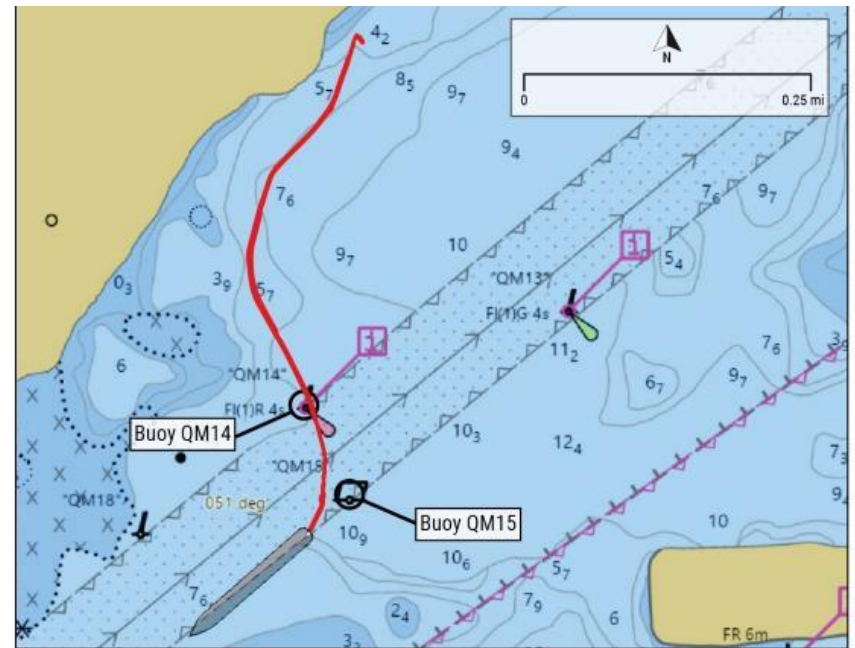
Figure 3. American Mariner's AIS path after it left the facility, in relation to the buoys, channel, and shoal water (final vessel position shown is at 0730:55). Soundings are in meters; shoal water is indicated with darker blue. (Background sources: Made Smart and NOAA)
