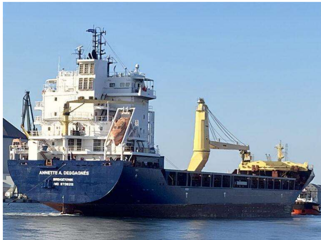
(Photo credits: Desgagnés photo of ice-class ANNETTE A. DESGAGNÉS multi-purpose vessel specially designed for heavy lift and project cargo)
