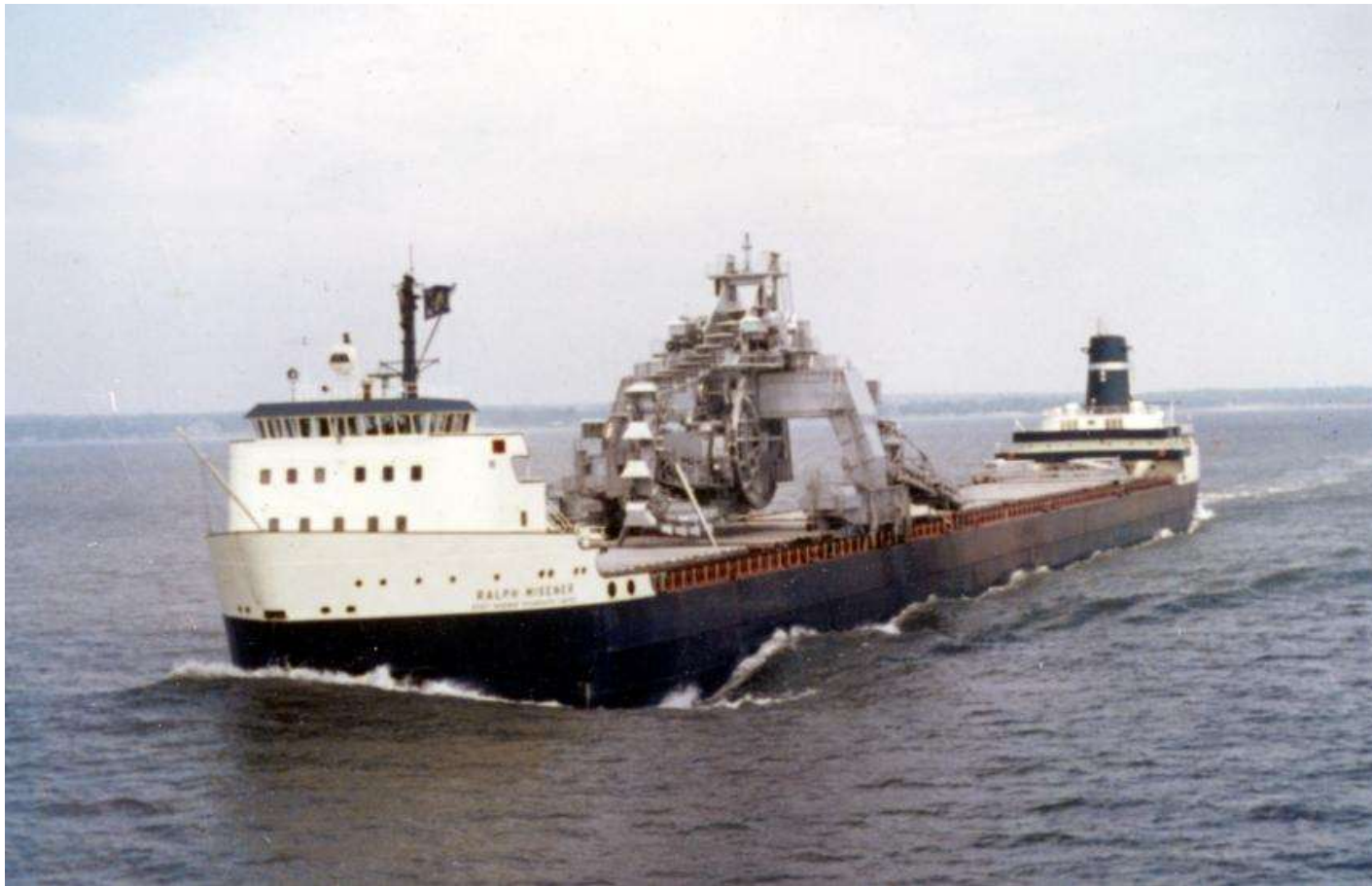
Ralph Misener with her unique Conflow self-unloading equipment on deck. [John Vournakis]
